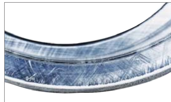
Fig. 34 Scoring on the Rib of Spherical Roller Bearing
