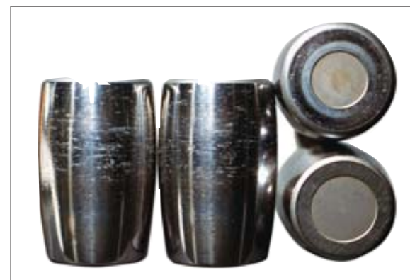
Fig. 35 Scoring on the Roller End Face
