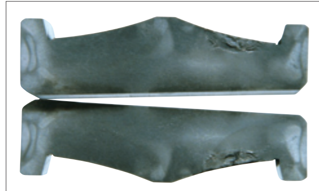
Photo 7-6-7 Part: Cross section of a fractured inner ring in Photo 7-6-6 Symptom: Origin is directly beneath the raceway surface
