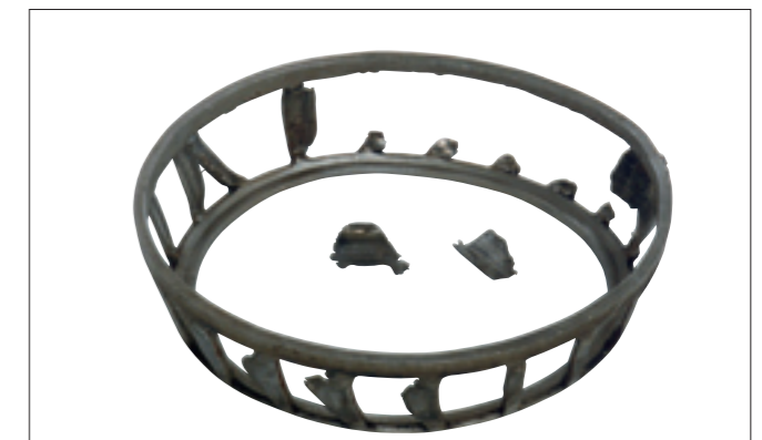
Photo 7-7-4 Part: Cage of a tapered roller bearing Symptom: Pillar fractures of pressed-steel cage
