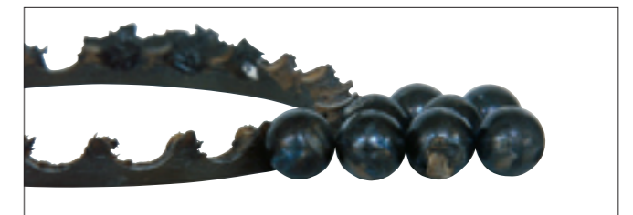
Photo 7-14-5 Part: Balls and cage of Photo 7-14-3 Symptom: Cage is damaged by melting, balls become discolored and melted Cause: Excessive preload
