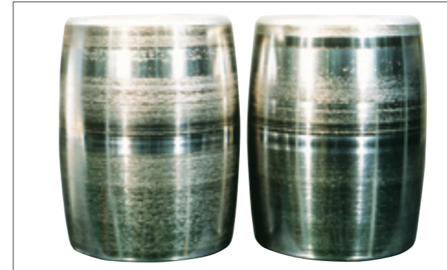
Photo 7-4-7 Part: Convex rollers of Photo 7-4-5 Symptom: Smearing occurs at the center of the rolling surface Cause: Poor lubrication
