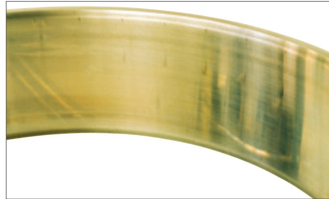
Photo 7-17-2 Part: Outer ring of a double-row cylindrical roller bearing Symptom: Axial scratches at roller pitch intervals on raceway surface Cause: Inclination of inner and outer rings during mounting
