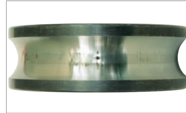
Photo 7-12-1 Part: Inner ring of a deep groove ball bearing Symptom: False brinelling occurs on the raceway Cause: Vibration from an external source while stationary
