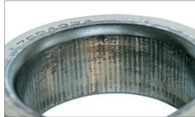
Photo 7-11-2 Part: Inner ring of an angular contact ball bearing Symptom: Notable fretting occurs over entire circumference of bore surface Cause: Insufficient interference fit
