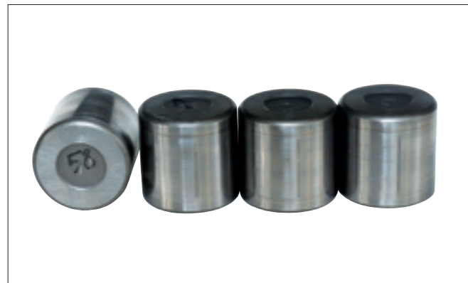
Photo 7-17-3 Part: Rollers of a cylindrical roller bearing Symptom: Axial scratches on rolling surface Cause: Inclination of inner and outer rings during mounting
