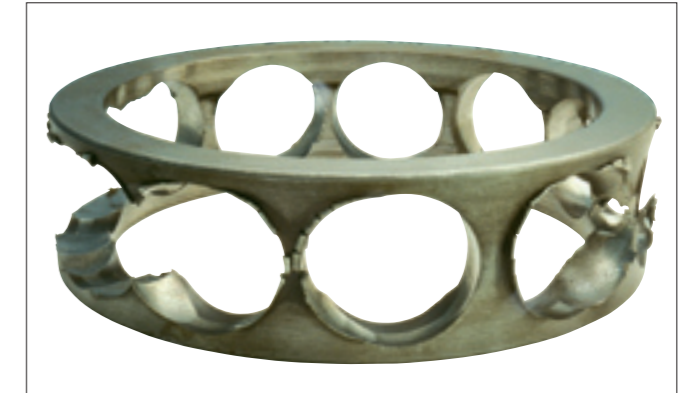
Photo 7-7-2 Part: Cage of an angular contact ball bearing Symptom: Pocket pillar fractures from a cast iron machined cage Cause: Abnormal load action on cage due to misaligned mounting between inner and outer rings
