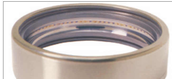
Photo 7-15-6 Part: Outer ring of a deep groove ball bearing Symptom: Fluting occurs on the raceway surface (High frequency)
