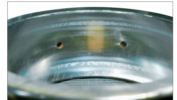
Photo 7-2-4 Part: Outer ring of a spherical roller bearing Symptom: Peeling occurs near the shoulder of the raceway over the entire circumference Cause: Poor lubrication
