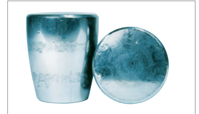
Photo 7-3-6 Part: Convex rollers of Photo 7-3-5 Symptom: Scoring on the roller end face Cause: Debris, which is caught in surface, and excessive axial loading
