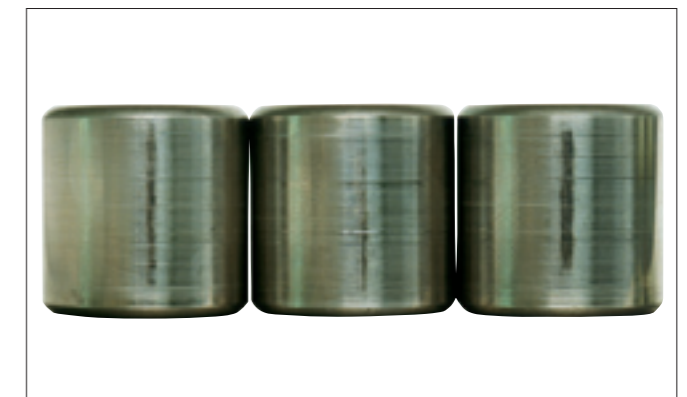
Photo 7-12-4 Part: Rollers of a cylindrical roller bearing Symptom: False brinelling occurs on rolling surface Cause: Vibration from an external source while stationary
