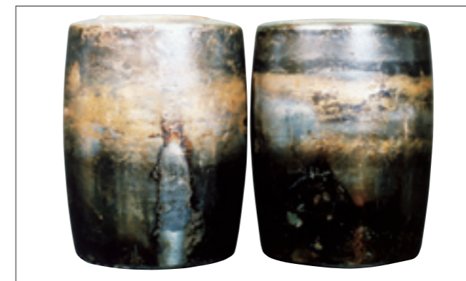
Photo 7-14-2 Part: Convex rollers of Photo 7-14-1 Symptom: Discoloration and melting of roller rolling surface, adhesion of worn particles from cage Cause: Insufficient lubrication
