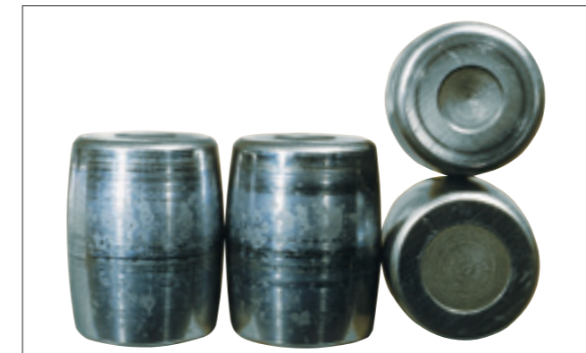
Photo 7-2-3 Part: Convex rollers of Photo 7-2-1 Symptom: Round shaped peeling pattern occurs on the center of the rolling surfaces Cause: Poor lubrication
