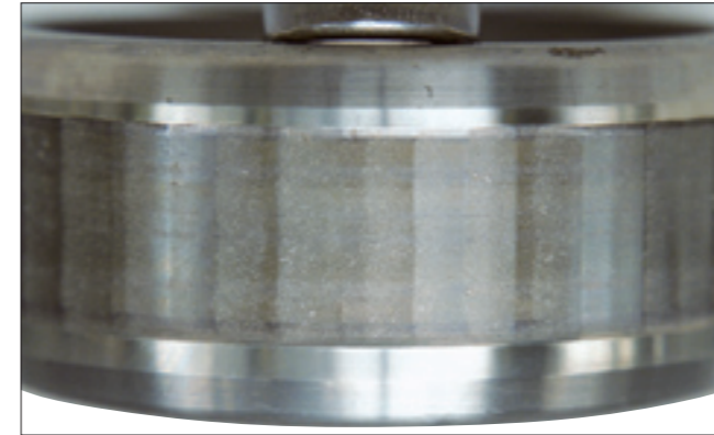
Photo 7-10-1 Part: Inner ring of a cylindrical roller bearing Symptom: Many pits occur due to electrical corrosion and wave-shaped wear on raceway surface Cause: Electrical corrosion
