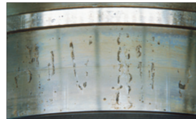
Photo 7-16-3 Part: Inner ring of a spherical roller bearing Symptom: Rust on raceway surface at roller pitch Cause: Entry of water into lubricant
