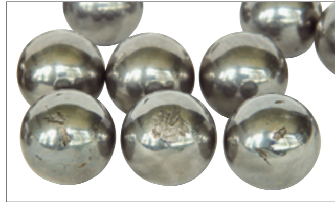
Photo 7-1-6 Part: Balls of Photo 7-1-4 Symptom: Flaking of ball surface Cause: Dents due to shock load while stationary
