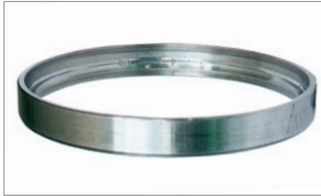
Photo 7-1-5 Part: Outer ring of Photo 7-1-4 Symptom: Flaking of raceway surface at ball pitch Cause: Dents due to shock load while stationary
