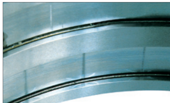
Photo 7-11-3 Part: Outer ring of a double-row cylindrical roller bearing Symptom: Fretting occurs on the raceway surface at roller pitch intervals
