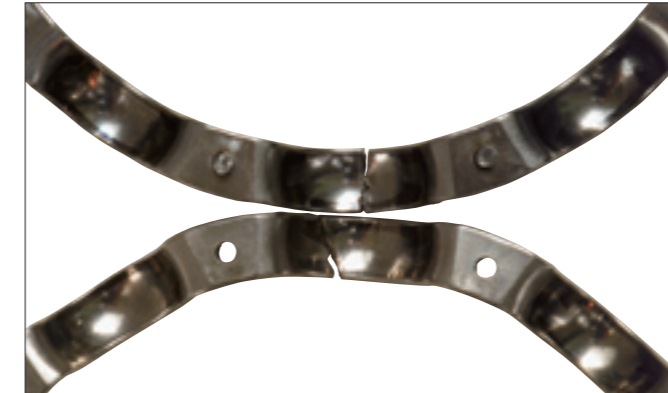
Photo 7-7-1 Part: Cage of a deep groove ball bearing Symptom: Fracture of pressed-steel cage-pocket
