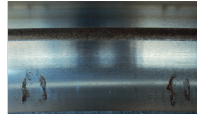
Photo 7-16-2 Part: Outer ring of a slewing ring Symptom: Rust on raceway surface at ball pitch Cause: Moisture condensation during stationary periods
