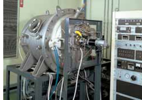
Photo 4.1 Vacuum testing system
