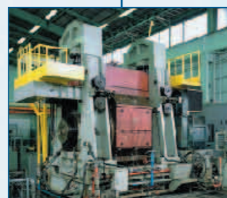
Tester for bearings used in backup rolls of rolling mills
