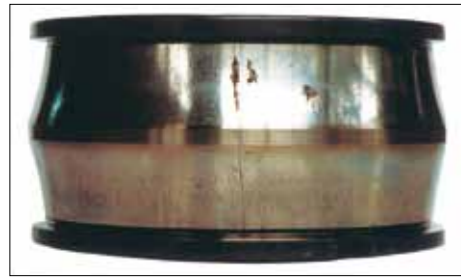
Inner ring fracture
